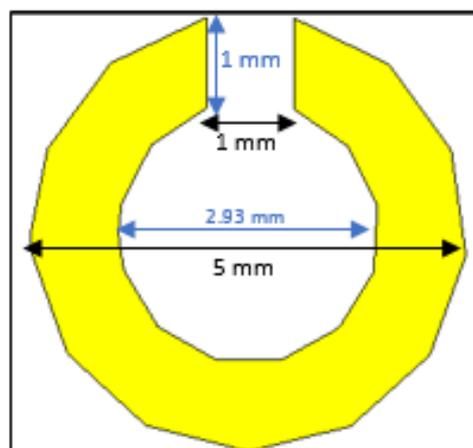
Figure 7. The size of ring metamaterial on vivaldi array antenna
