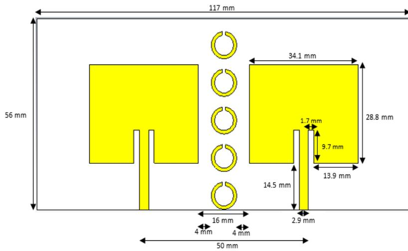
Figure 3. Square array antenna with ring metamaterial
