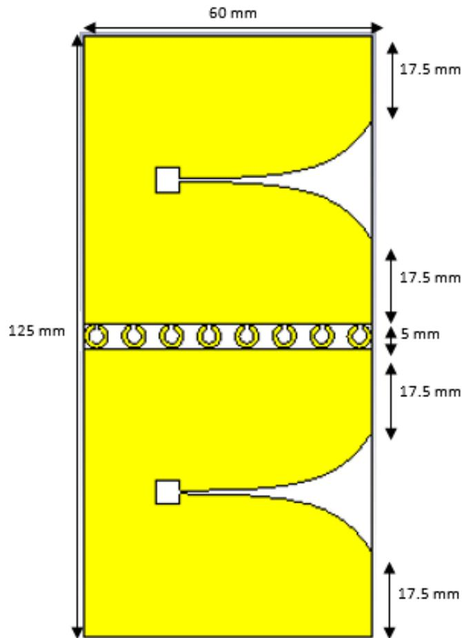
Figure 6. Vivaldi array antenna with ring metamaterial
