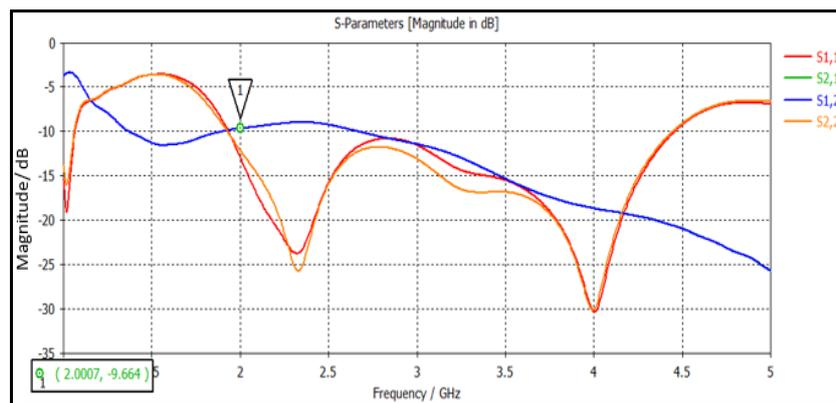
Figure 10. S-Parameter of vivaldi array antenna without metamaterial
