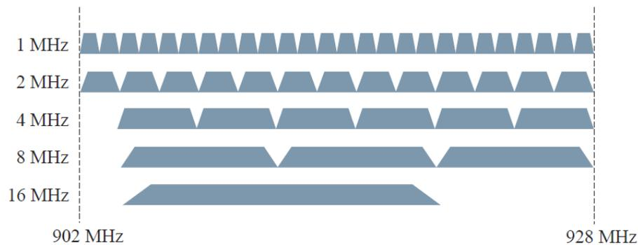
Figure 2. IEEE 802.11ah channelization (Sun et al., 2017)
