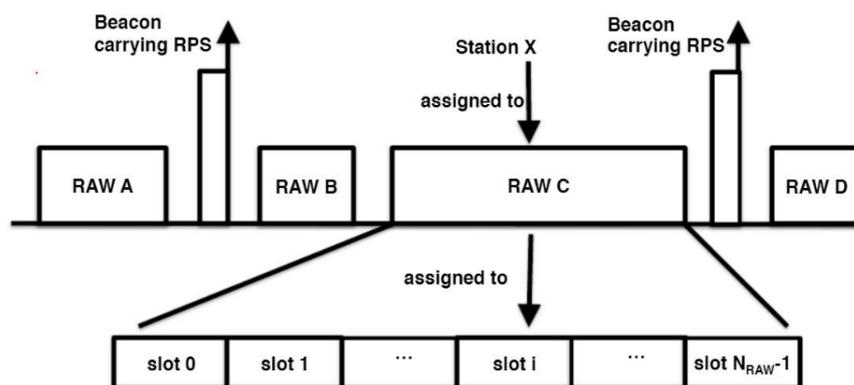
Figure 4. RAW Mechanism (Tian, Deronne, et al., 2016)
