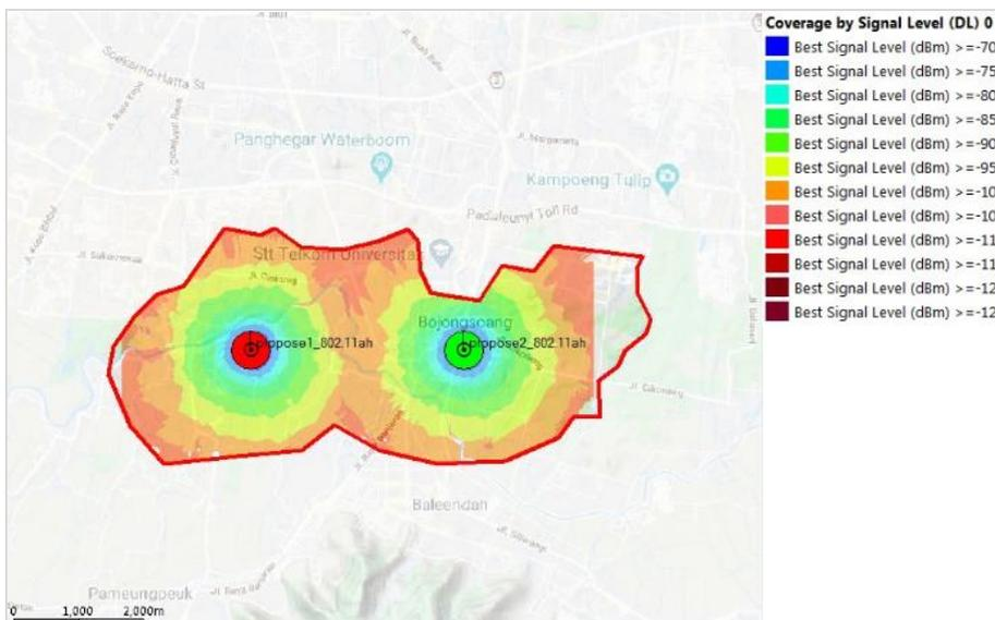
Figure 20. 802.11ah fills Suburban LTE Blank spot area
